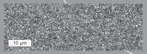
> **Submicron grain cemented carbides** are our most frequently used grain size class. The very homogeneous, fine microstructure of this grade allows for high hardness and cutting abilities and is excellently suited for machining and milling tools, drills, guides, cutting tools, pressing dies, in wear protection and even for fine punching tools.
