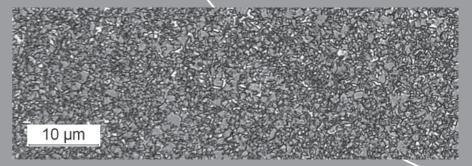
These cemented carbide grades with medium grain size combine good hardness and wear resistance with high transverse rupture strength, fracture toughness and thermal shock resistance. Application in general wear protection, for guides, bushings, slide rings, cutting rings, blades, lathe tips, reshaping, rolling, drawing and pressing tools.
